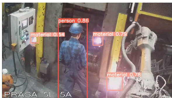
Fig. 2. Network performance in the known environment with a confidence threshold of 0.5
