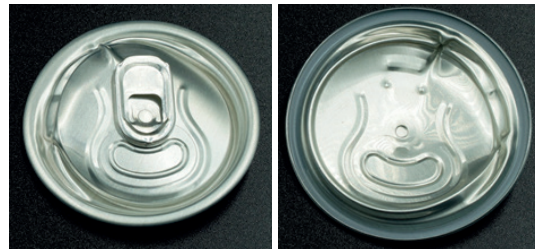
Fig. 5. Beverage can end after the buckling test
