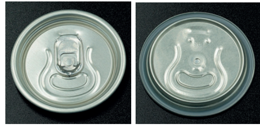
Fig. 4. Beverage can end before the buckling test
