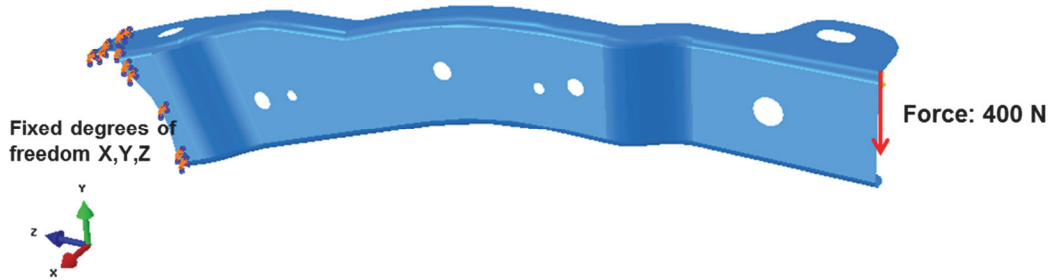
Fig. 5. Illustration of the numerical test performed to evaluate stiffness of the bracket.
