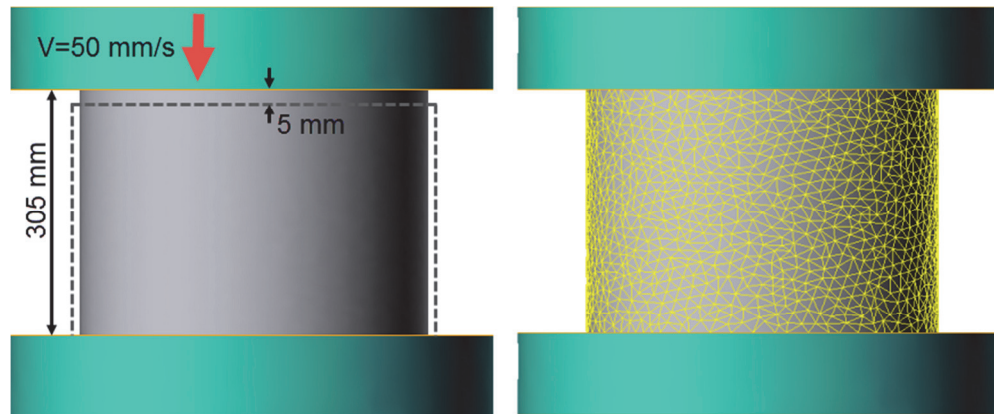
Fig. 2. Scheme of upsetting (left) and finite element mesh with element size of 20 mm (right)
